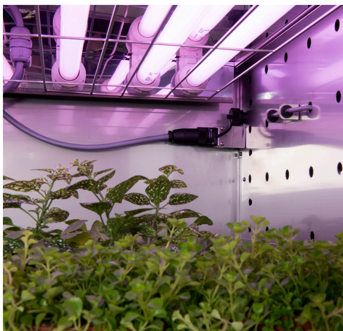
Interior of Thermo Scientific Vertical Light Chamber with plant growth light modules installed.
