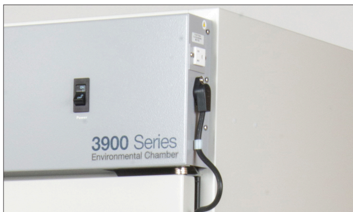
Exterior receptacle, located on the upper-right side of the control panel, is available for connecting an optional recorder or other Thermo Scientific accessories.
