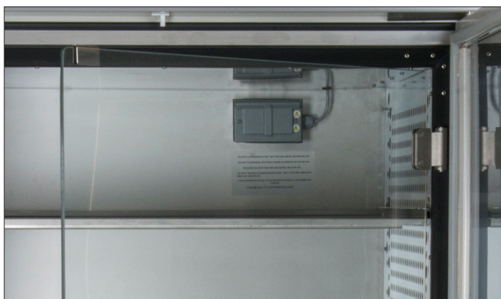
Interior GFCI receptacle located in the upper right corner of the rear wall, permits the use of shakers, cell rollers, and other equipment inside the chamber, eliminating the inconvenience of an extra external power strip.
