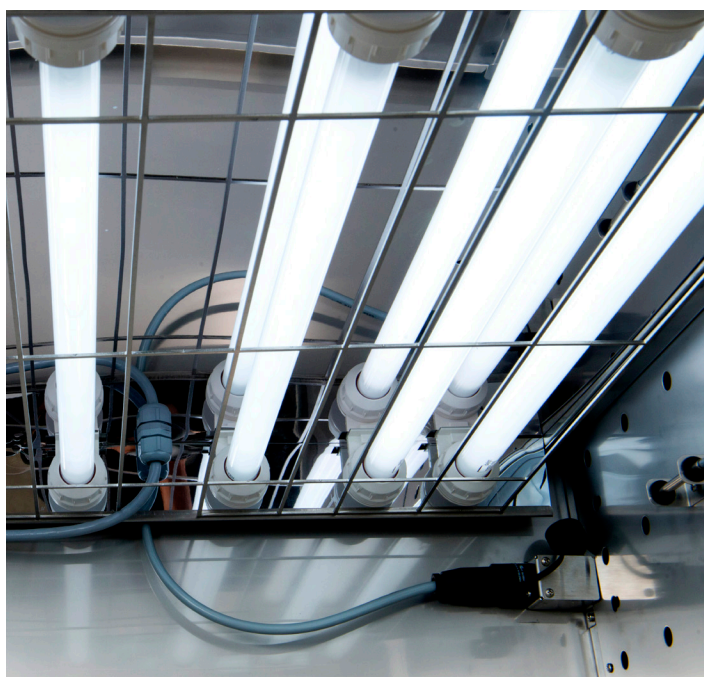
Interior of Thermo Scientific Vertical Light Chamber with animal hatching light modules installed.
